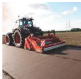
LRP Profi with Hydr. adjustable roller
