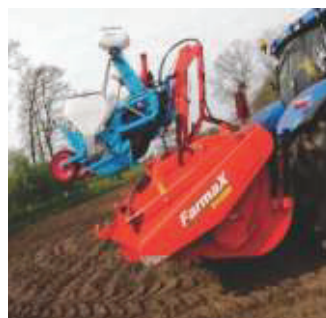
LRP Profi with rotary harrow and hydr. lift
