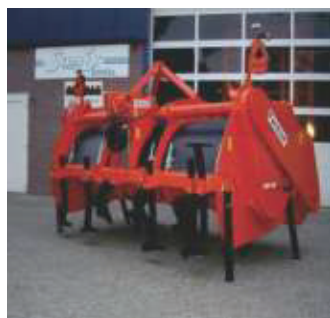
LRP Profi with rotary harrow and coulters
